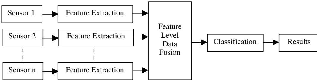
Figure 2. Feature level multisensor image fusion procedure
