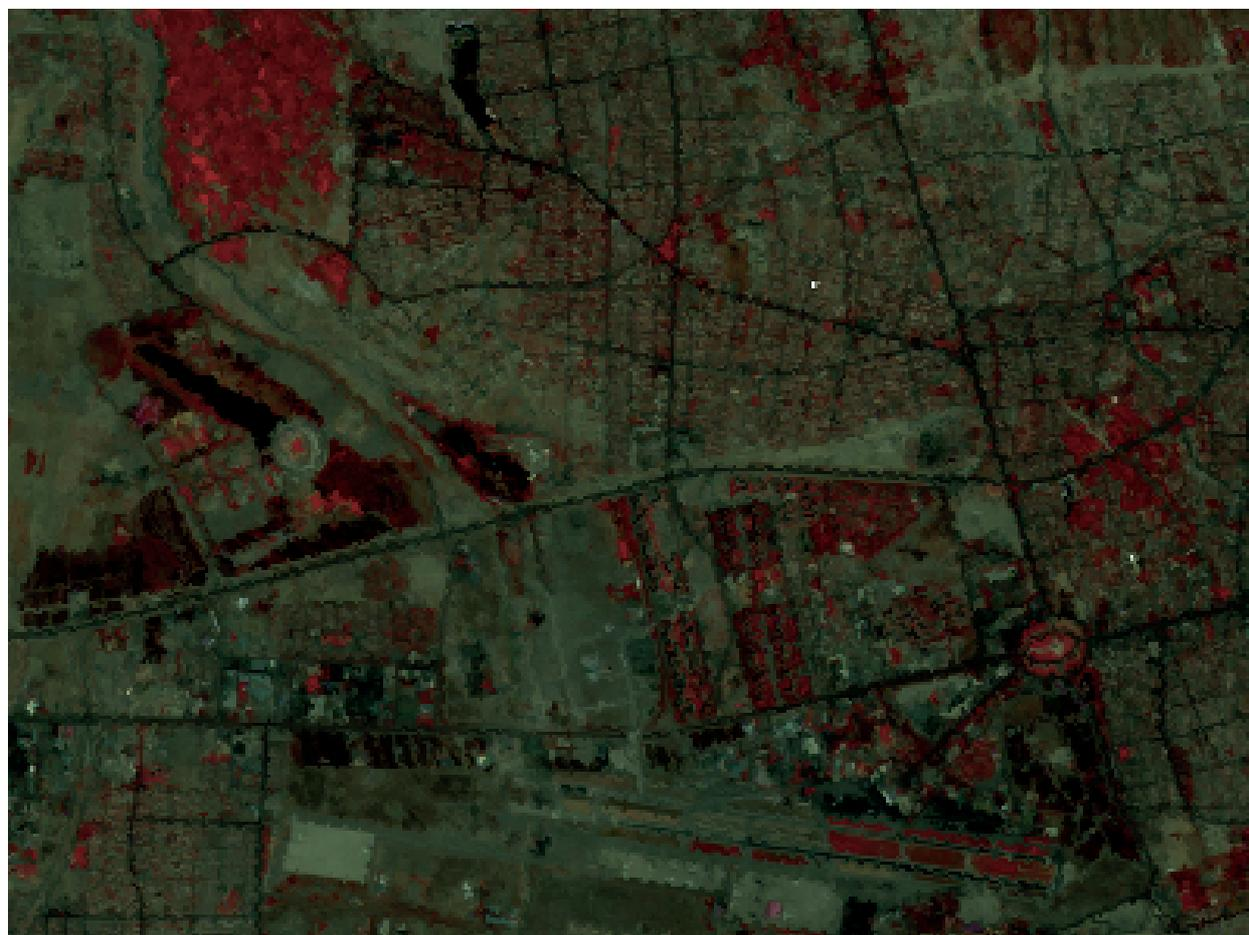
Figure 6. RGB color composite image of the original 4,3,2 TM bands, with 30-m spatial resolution
