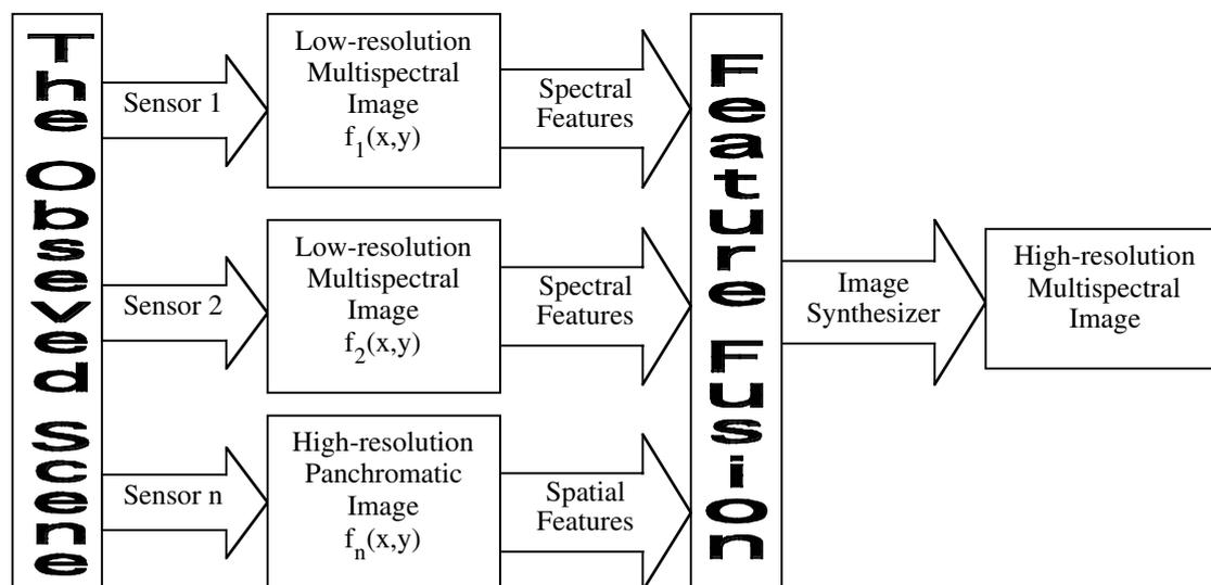
Figure 5. Multisensor image data fusion by the spatial-spectral feature synthesizer
