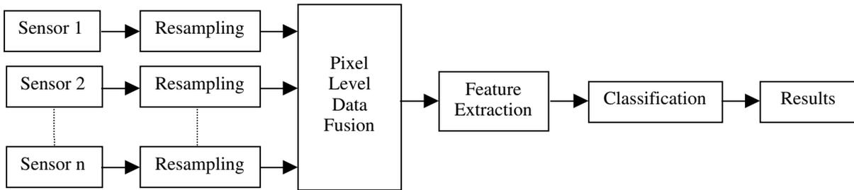
Figure 1. Pixel level multisensor image fusion procedure
