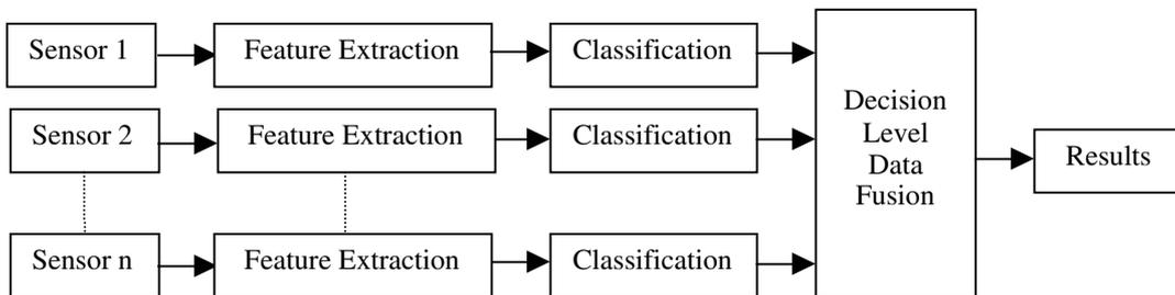
Figure 3. Decision level multisensor image fusion procedure
