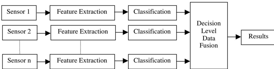
Figure 3. Decision level multisensor image fusion procedure
