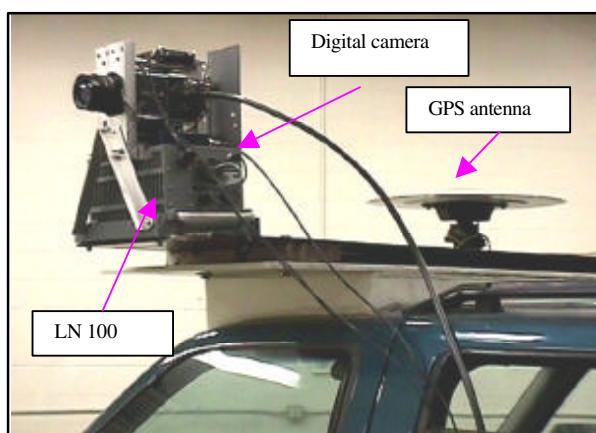
**Figure 2.** GPS/INS/CCD hardware configuration.
