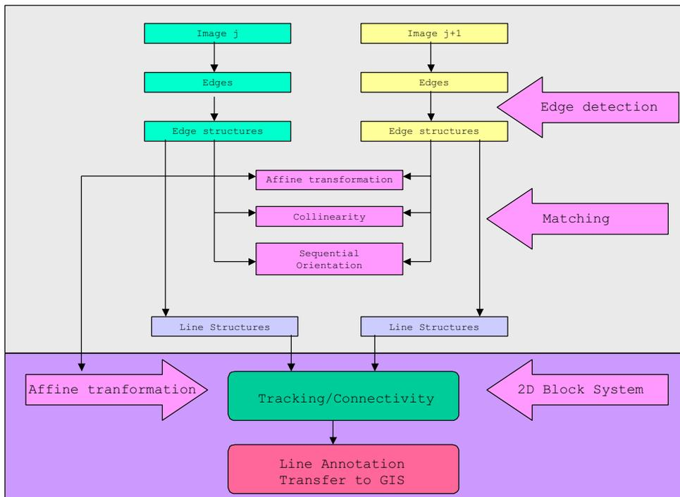
Figure 1. Image processing concept (top block: real-time, lower block: post-processing).
