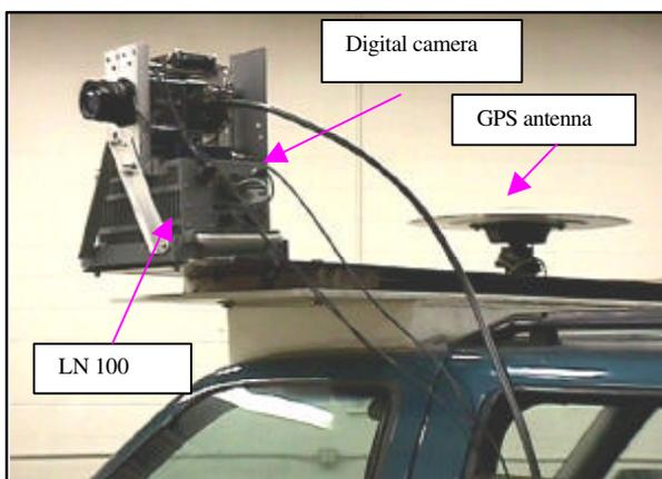
Figure 2. GPS/INS/CCD hardware configuration.
