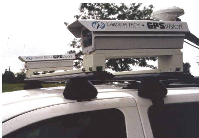
Fig. 1 Portable GPSVision system consists of GPS, INS and Digital Cameras
