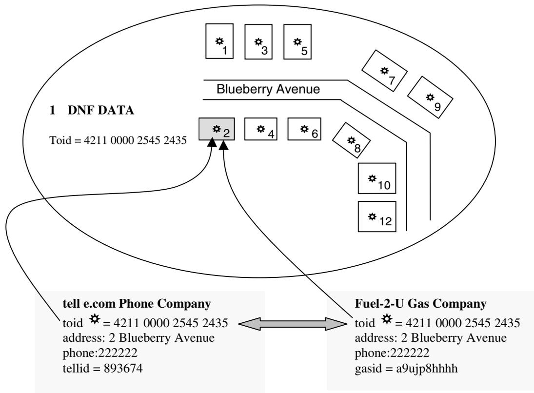
Figure 1: Many users can reference the same feature using the Topographic Object Identifier (TOID). They will be able to access change information from DNF on each feature they hold. They can also unambiguously share information about features they hold in common.
