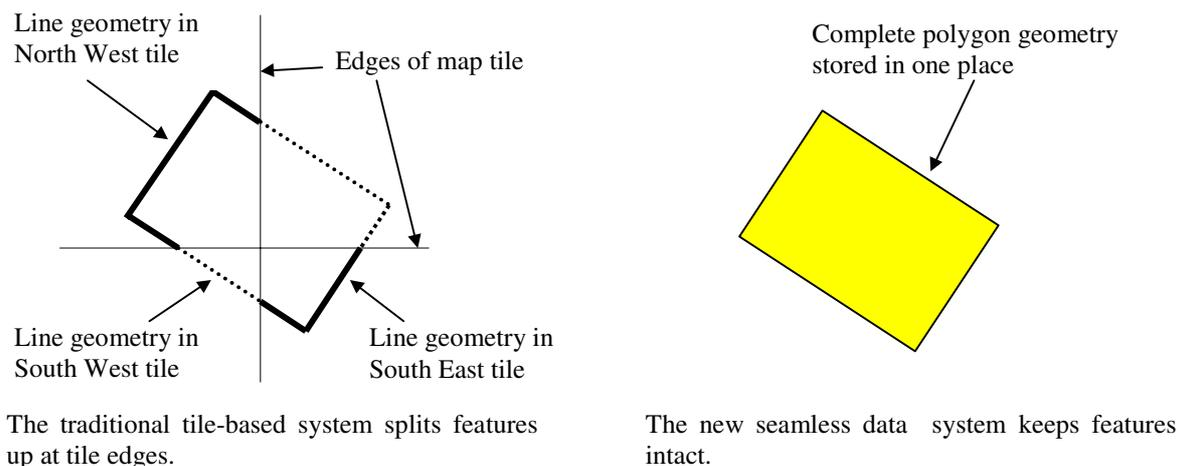
Figure 2: Polygons crossing tile edges in the old system will be retained as single objects in DNF.
