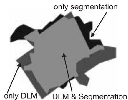
Figure 5: Result of corresponding disjoint objects (lightgray: DLM- and image object; gray: only DLM object; darkgrey: only image object)
