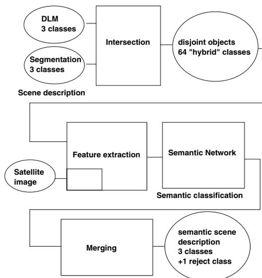
Figure 3: Flowchart of the integrated analysis of image and DLM.
