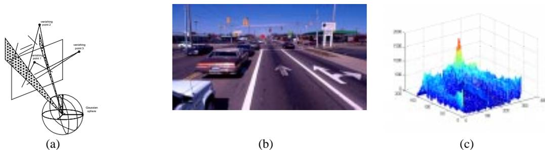
Figure 5. Vanishing points detection algorithm applied in both the color image and gray image, (a) Vanishing point geometry and the corresponding Gaussian sphere, (b) A color image of size 720X400, (c) Voting space of  $(\theta_u, \phi_u)$  generated from the straight lines extracted in (b).
