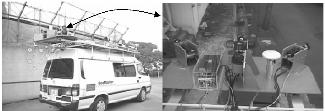
Figure 1. Mobile Mapping Survey Vehicle and the Sensors on top of the vehicle
