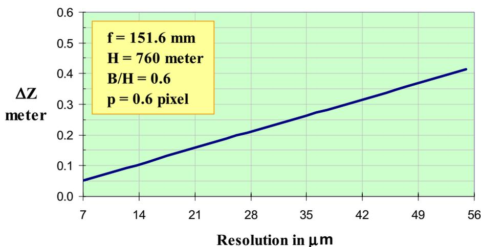
Figure 1. Theoretical Values of  $\Delta \mathbf{Z}$  for Generated Surface at Various Resolutions
