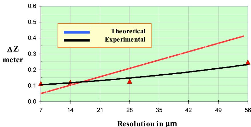
Figure 3. Experimental values of  $\Delta Z$  compared to theoretical values
