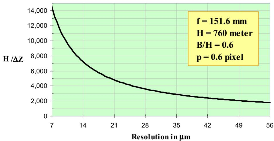
Figure 2. Theoretical Values of  $H/\Delta Z$  Based on Various Resolutions.
