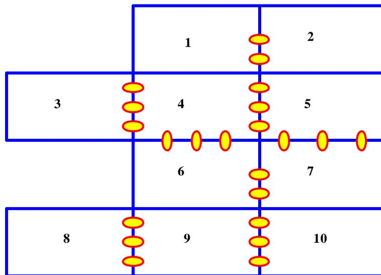
**Figure (2) Layout of Ortho-sheets and measured distances.**
