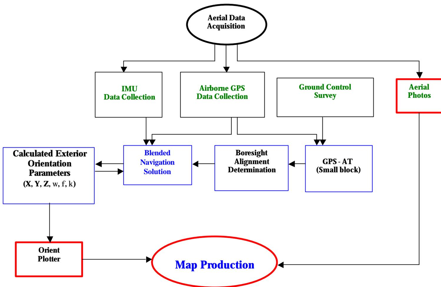
Figure (1) Flowchart of the IMU/map production process Table (1) Results of Ground Control Points in Fayette County
