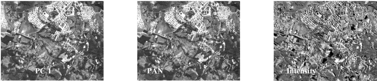
The hybrids images are submitted to a segmentation process which consists of ISODATA clustering. This method uses spectral distance in the sequential way, but iteratively classifies the pixels, redefines the criteria for each segment, and classify again, so that the spectral distance patterns in the data gradually emerge.
