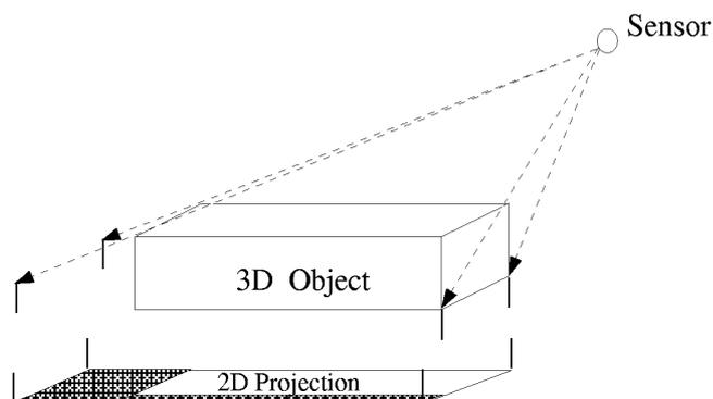
Figure 3: A model of perspective distortion.
