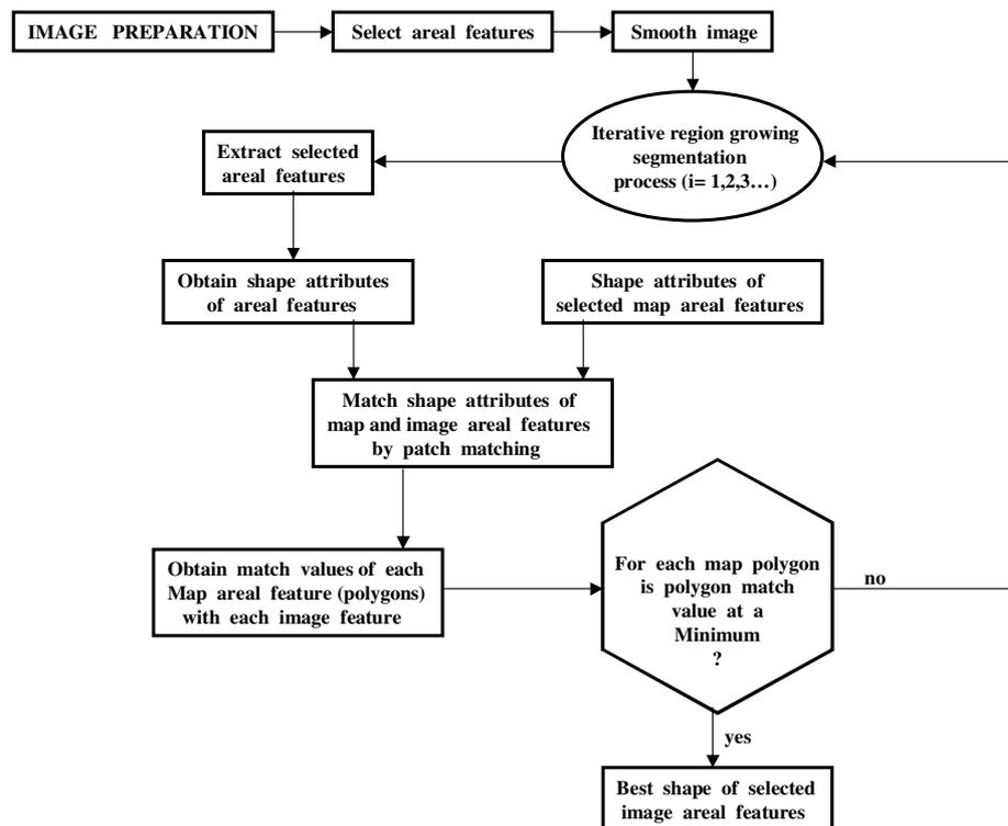
Figure 2: Algorithm for extracting selected image features with best shape.
