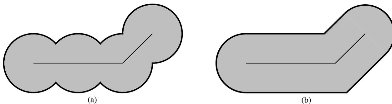
Figure 2: Search area formed along a polygon by point buffers (a) and search area formed by a polygon buffer (b).
