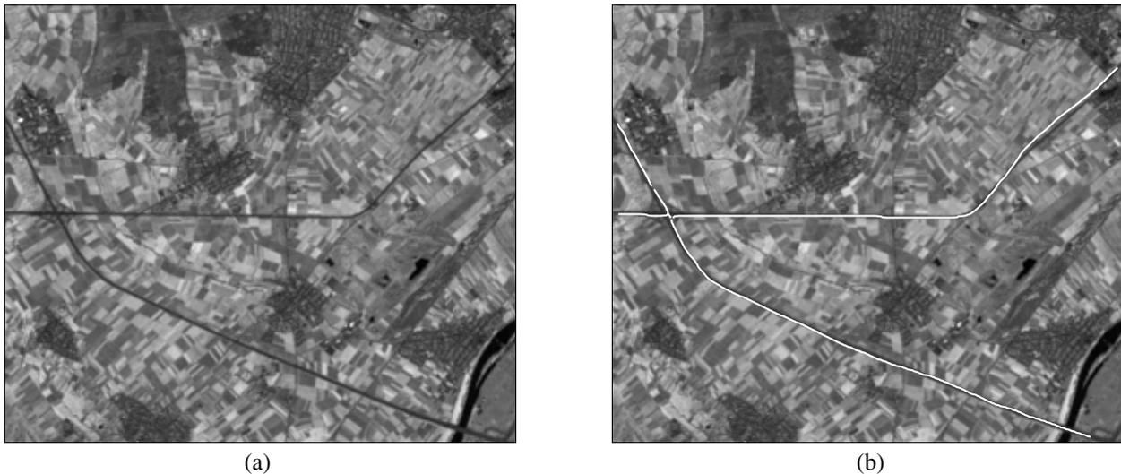
Figure 6: IRS-1C data, ground resolution  $23\text{ m} \times 23\text{ m}$  (a), and IRS-1C data with motorways from GIS (b).
