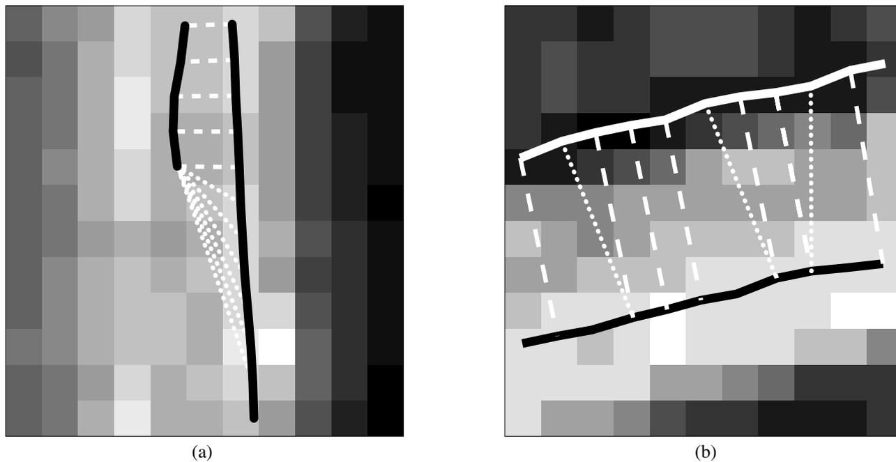
Figure 4: Effects of back-checking. The thick solid lines represent GIS objects and images features. The dashed lines stand for the matches remaining after back-checking and the dotted lines are the matches eliminated by back-checking. The black and white colours have been chosen for reasons of contrast only.
