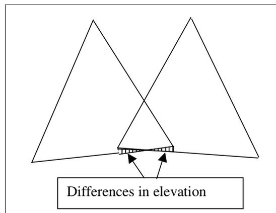
Figure 1 Misalignment in roll causes discrepancies between strip also in flat areas.
