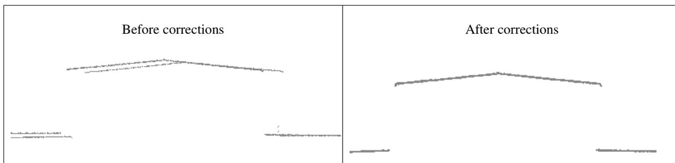
Figure 7 Profiles of the building in test area 2 (two laser strips in opposite directions) before and after correction of orientation errors.
