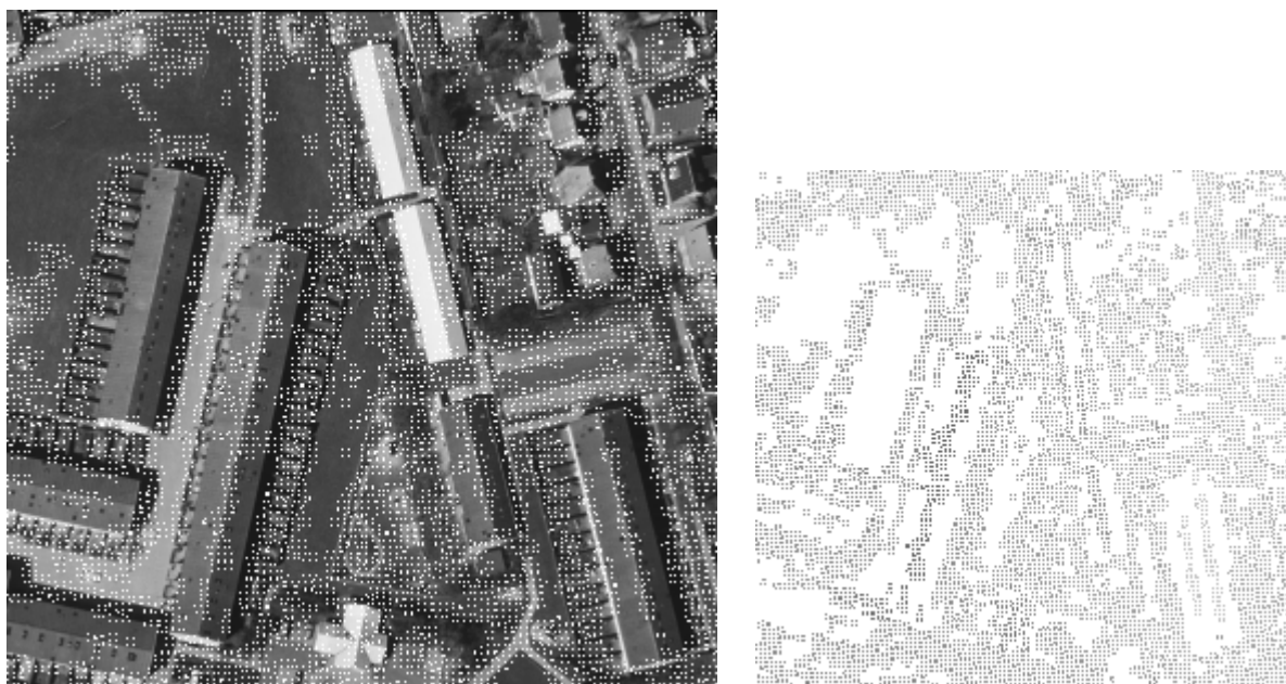
Figure 1. The dots represent the places with Z value generated in the automatic process of DEM generation: on the left- white dots are projected on the left image, on the right- black dots are projected on XY plane of the object space with scale dependent of size of user window and original image pixel size.
