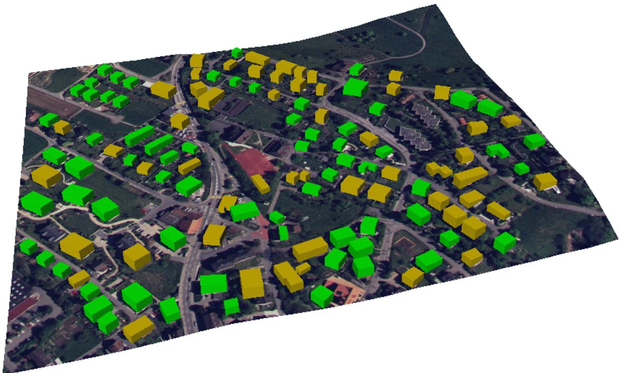
Figure 4. Reconstructed buildings. The colours green (darker) and yellow (lighter) indicate different degree of reliability. Green buildings were accepted automatically, yellow after manual inspection (but no editing).
