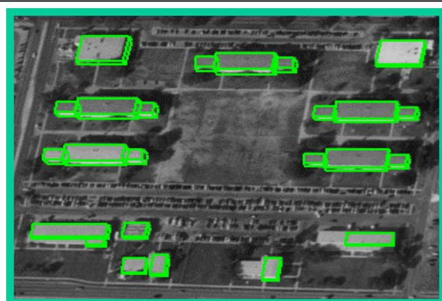
Figure 24. Building components extracted using DEM cues
