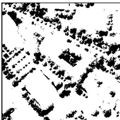
Figure 3: Segmented vegetation areas by means of NDVI
