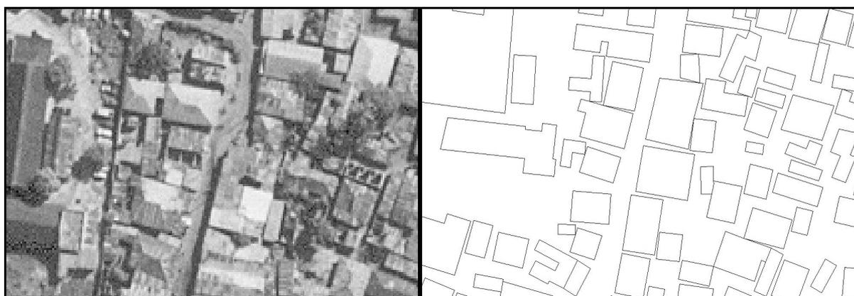
Figure 2. Left: exert of 1992 aerial photograph (Original scale 1:12500). Note the high density, irregular distribution of buildings and the highly generalised building forms. Right: exert of building polygon coverage after processing.
