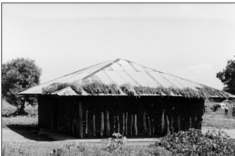
Figure 1. Small building that yielded a strong reflection on the SAR image because of the specific orientation of the corrugated iron roof (mirror-effect).
