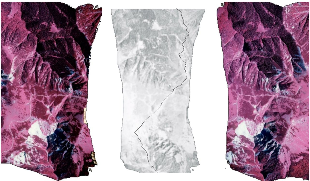
Figure 7: Orthophotos 7472 (left), 7468 (right) and the image representing the photometric energy terms in the overlap area (middle): the darker the image, the higher the energy. The displayed line is the seam line as proposed by the algorithm.
