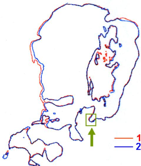
Figure 2. Changes in position of Aral Sea coastline derived using channel 2 of AVHRR. 1 is for May 1997, 2 is for May 1996.
