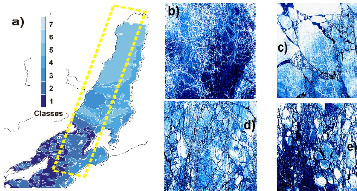
Figure 4. May 18, 1999, (a) the distribution of classes of underlying surface for a multispectral picture from AVHRR, and the correspondence of some of the classes and types of ice identified in the image in MSU-E channel 2: (b) class 2, (c) class 3, (d) class 4, (e) class 5.
