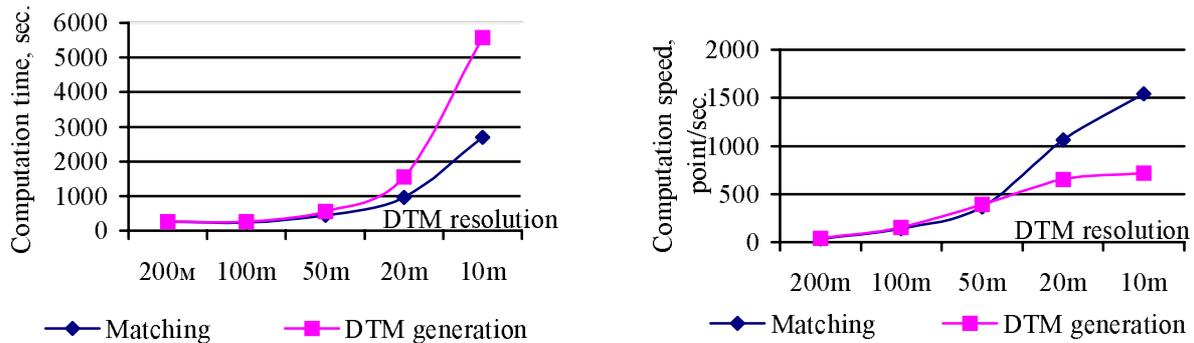
Figure 10. Temporal performances of the hierarchical DTM generation method
