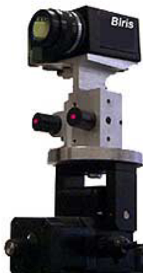
Figure 1. The Long Range Biris sensor
