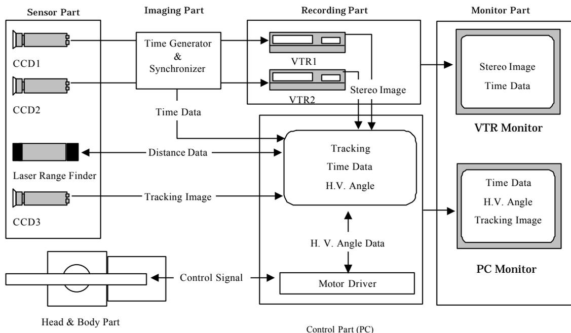
Figure 1. System configuration of HVT system
