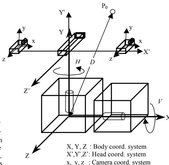
Figure 4. Coordinate system of HVT
