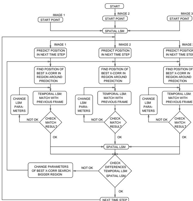
Figure 7. Flowchart of the LSM tracking process
