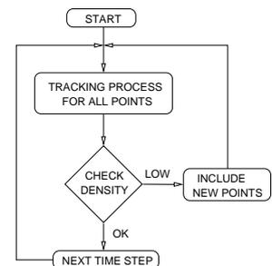
Figure 9. Flowchart of the surface tracking process
