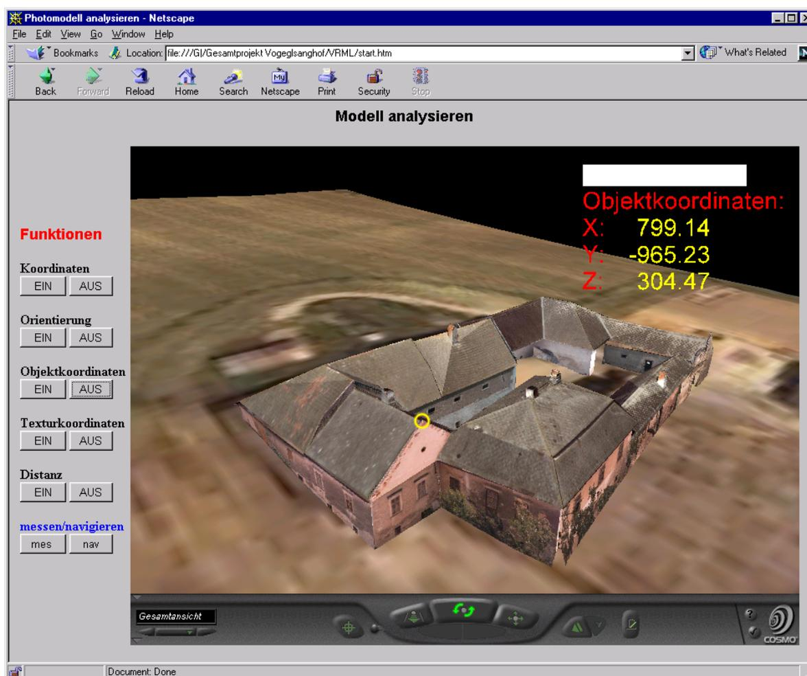
Figure 4. VRML visualisation and co-ordinate measurement tools using the EAI.
