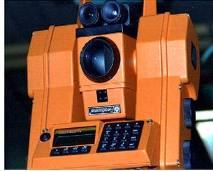
Fig. 2: Image acquisition unit.
