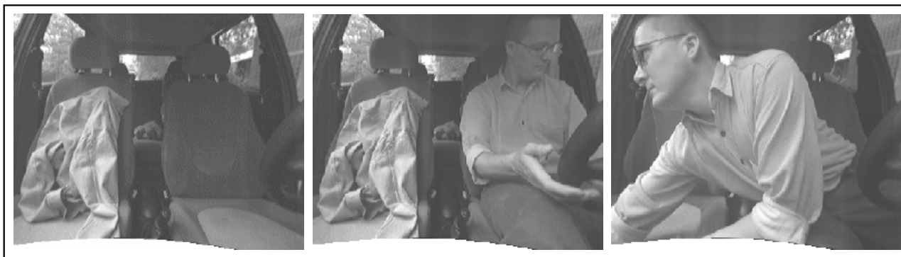
Figure 1: Possible scenarios seen by a camera inside a vehicle, which are of special interest for an intelligent airbag deployment.
