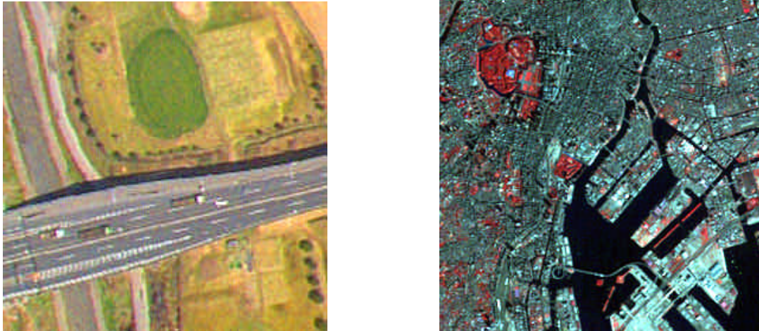
(a) High Resolution Image (Aerial HDTV Image, 30cm) (b) Usual Satellite's Image (LANDSAT TM, 30m) Figure 1: Comparison of High Resolution Image with Ordinary Satellite's Image.
