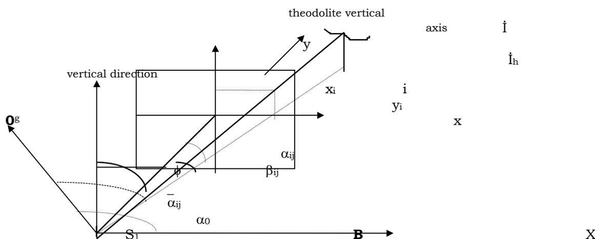
Figure 1. The relationship between the theodolite image coordinates and the horizontal and the vertical angles
