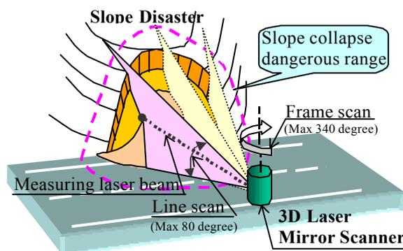
Fig. 6: Measurement system
