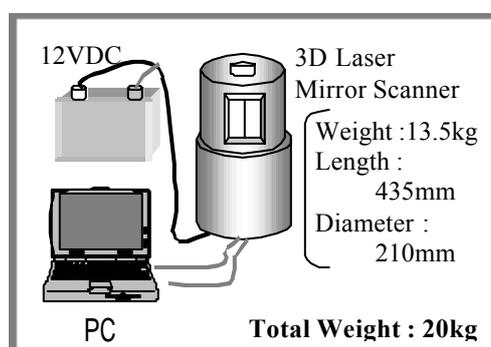
Fig-5 composition of measurement device
