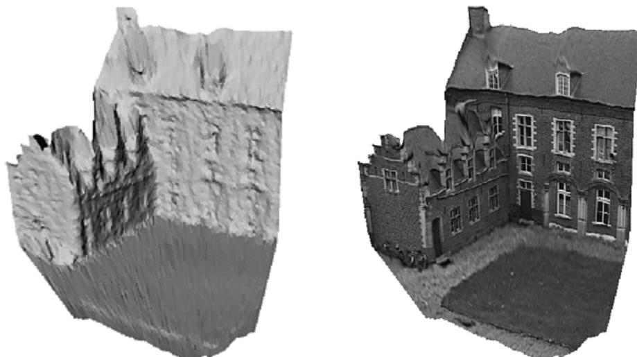
Figure 6: 3D surface model obtained automatically from an uncalibrated image sequence, shaded (left), textured (right).
