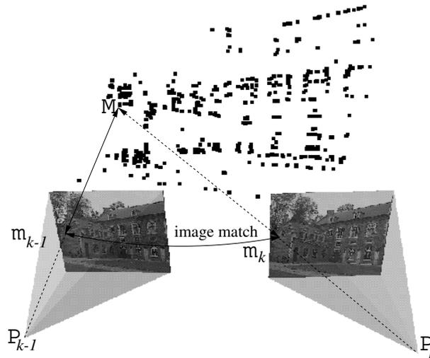
Figure 2: Image matches ( $m_{k-1}$ ,  $m_k$ ) are found as described before. Since the image points,  $m_{k-1}$ , relate to object points,  $M_k$ , the pose for view  $k$  can be computed from the inferred matches ( $M$ ,  $m_k$ ).
