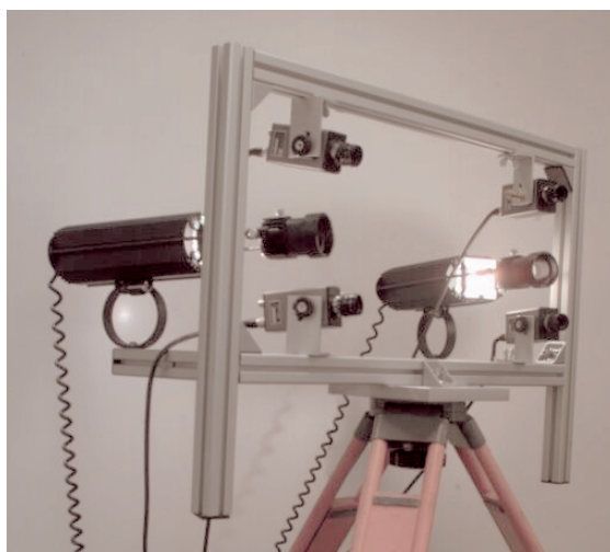
Figure 1. Set-up with video cameras and projectors
