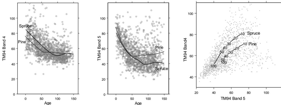
Figure 3. a) Scatterplot of TM band 4 (1994) vs age with Loess interpolation for pine- and spruce-dominated sample plots. b) same with TM band 5. c) Band 4-5 spectral space with the Loess interpolations from a) and b) plotted against all pixel values in background.
