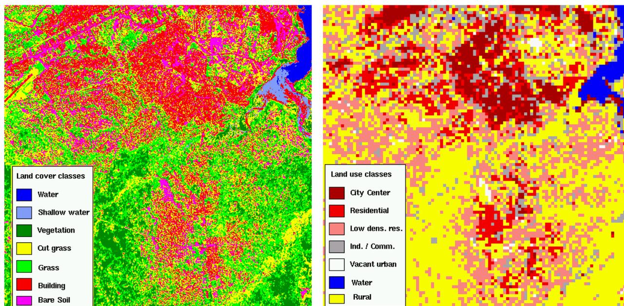
Figure 4: Two-stage classification: land cover(left) and land use, derived from land cover densities in  $5 \times 5$  cells (right).
