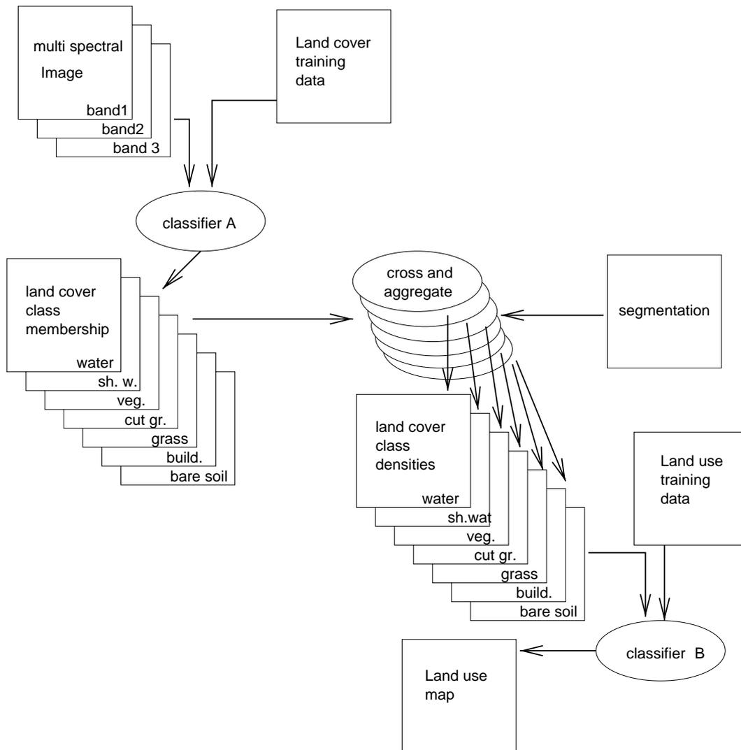
Figure 3: Two-stage classification flow diagram
