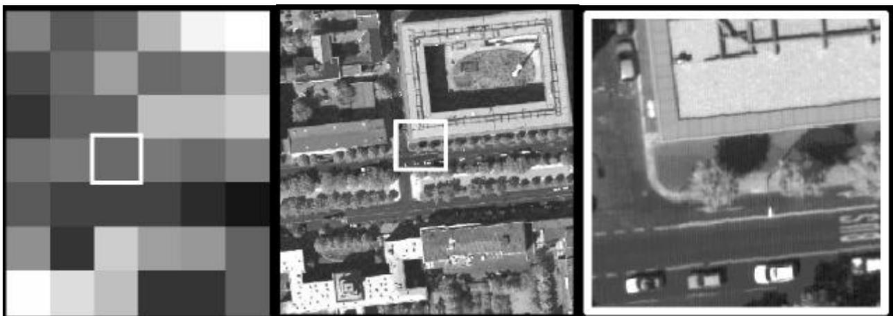
Figure 1. A demonstration of the issues surrounding the spatial resolution of different instruments. Left to right: Landsat TM 30 m data, HRSC-A 30 cm data with TM pixel identified, HRSC-A 30 cm data of the TM pixel enlarged.
