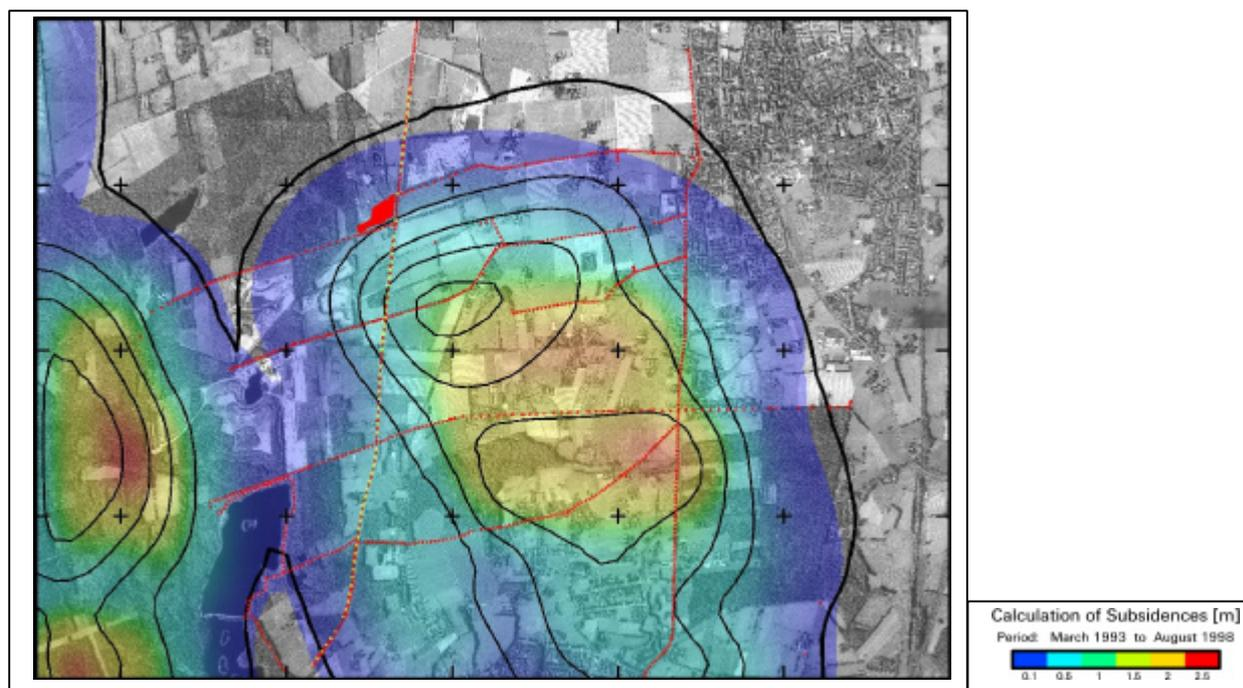
Fig. 2: HRSC-A orthoimage August 1998; "Calculation of Subsidence 1993-1998";
