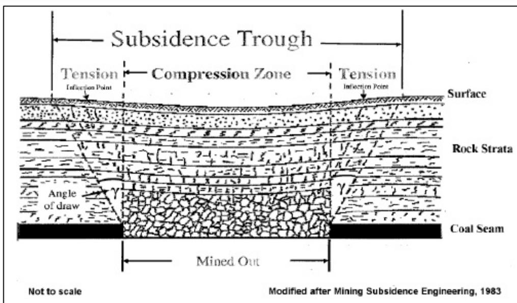
Fig. 1: Cross-section of subsidence trough
