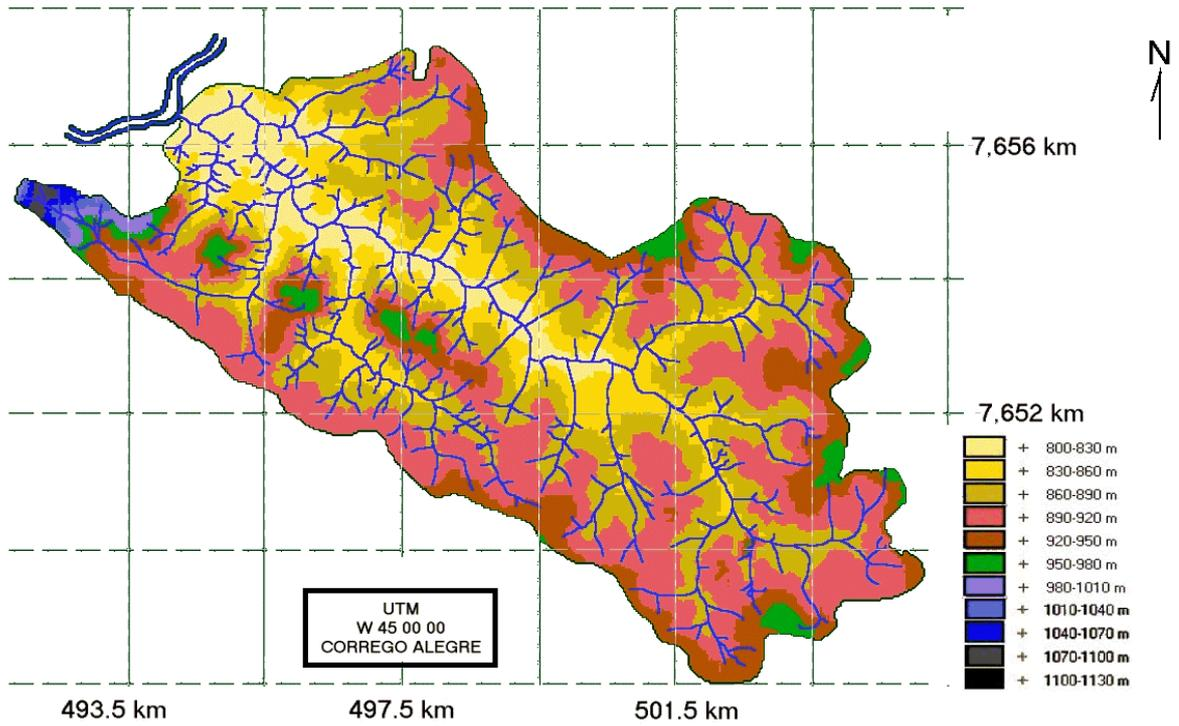
Figure 1: Hypsometric and drainage network of the Ribeirão Vermelho watershed
