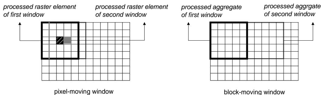
Figure 2: Two types of focal operators (for a window size of 5 x 5 pixels)
