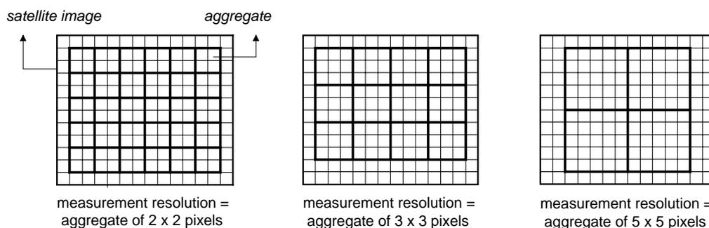
Figure 1: Example of an aggregate set, where  $s = \{2 \times 2, 3 \times 3, 5 \times 5\}$  spatial pixel blocks
