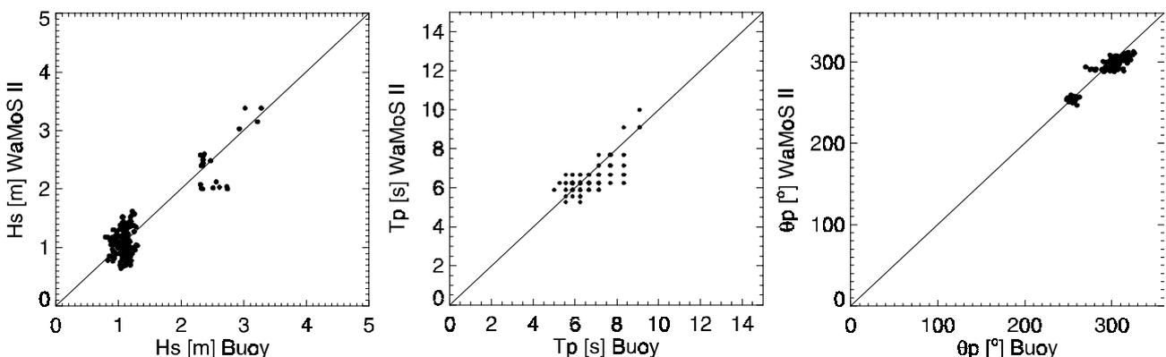
Figure 5. Scatter plots of buoy measurements versus radar results for significant wave height (left panel), peak wave period (centre panel), and peak wave direction (right panel).
