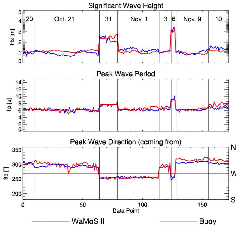
Figure 4. Significant wave height (upper panel), peak wave period (middle panel) and peak wave direction (lower panel) measured at Petten with WaMoS II (blue curves) and with a Directional Waverider (red curves). The figure covers only the periods during which the radar was switched on.
