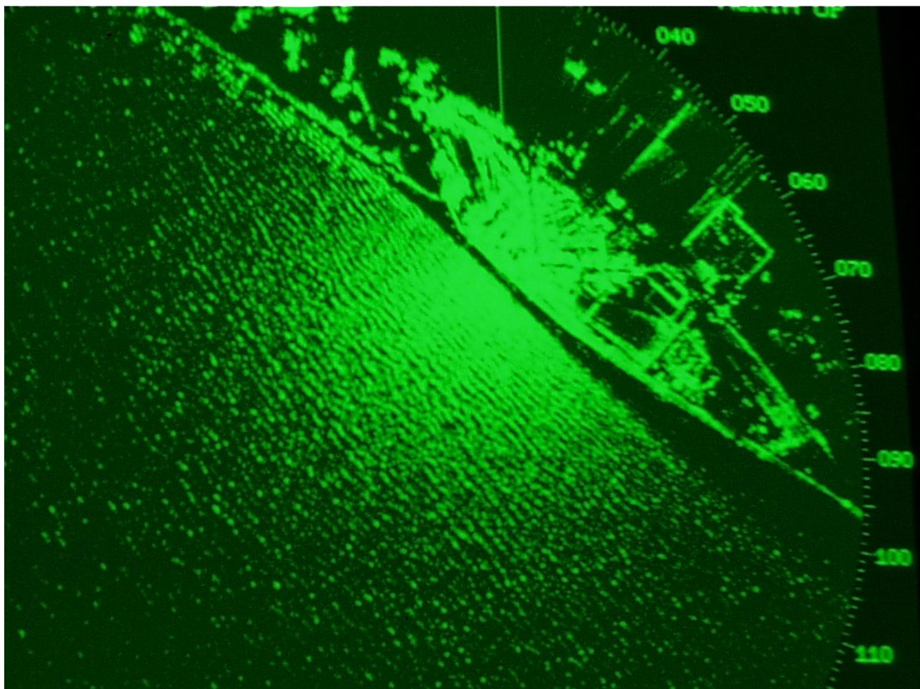
Figure 1. Part of a PPI image recorded at the Dutch coast near Petten, The coast line is from upper left to lower right. The direction scale at the edge of the PPI is partly visible. The wave pattern is clearly visible, and refraction may be seen near the shore. The image covers a few km.
