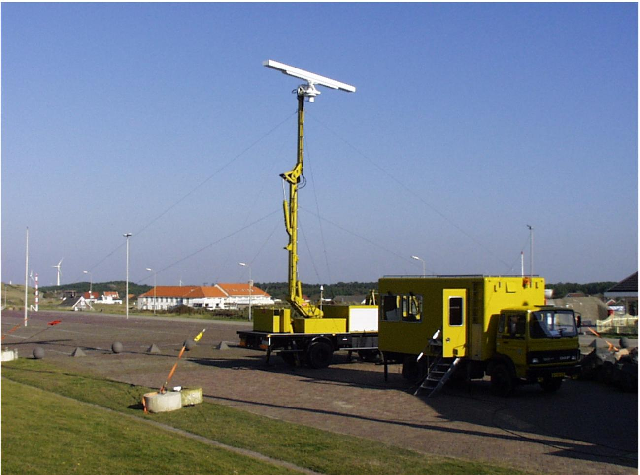
Figure 2. The mobile radar behind the dike at Petten. The photograph is taken from the landward face of the dike. The truck with the control cabin (right) partly blocks the sight of the truck with the antenna mount (left).
