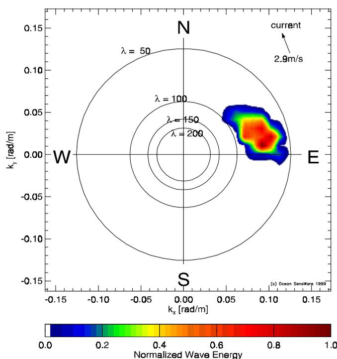
Figure 3. Two dimensional wave energy spectrum recorded with the mobile radar and WaMoS at Petten on October 31, 1999, 8:38 UTC. The spectrum has been normalised to one by the plotting software in order to cover the full colour scale.
