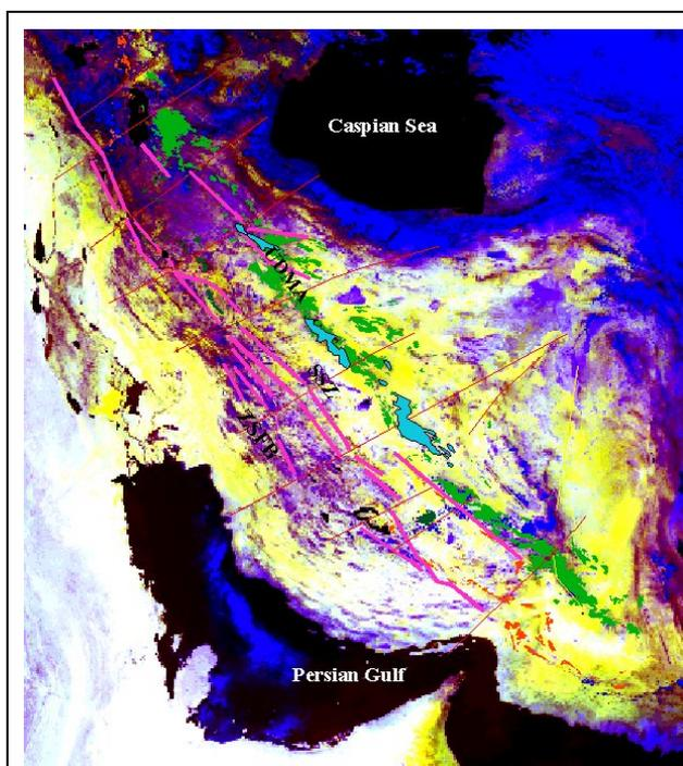
Figure 2. Colour composite AVHRR image (bands 4,3 and 2) with the overlaid maps of interpreted major faults, trending in a NW-SE (purple lines) and in NE-SW (red lines), and the interpreted magmatic rocks of UDMA arc (blue) along the axes of known magmatic rocks (green).
