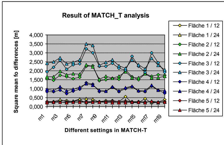
Figure 3. Statistical Analysis of the Elevation Accuracy in Dependence on the Scan Resolution (12 or 24  $\mu\text{m}$ ) and Topography (area1 – area 5)
