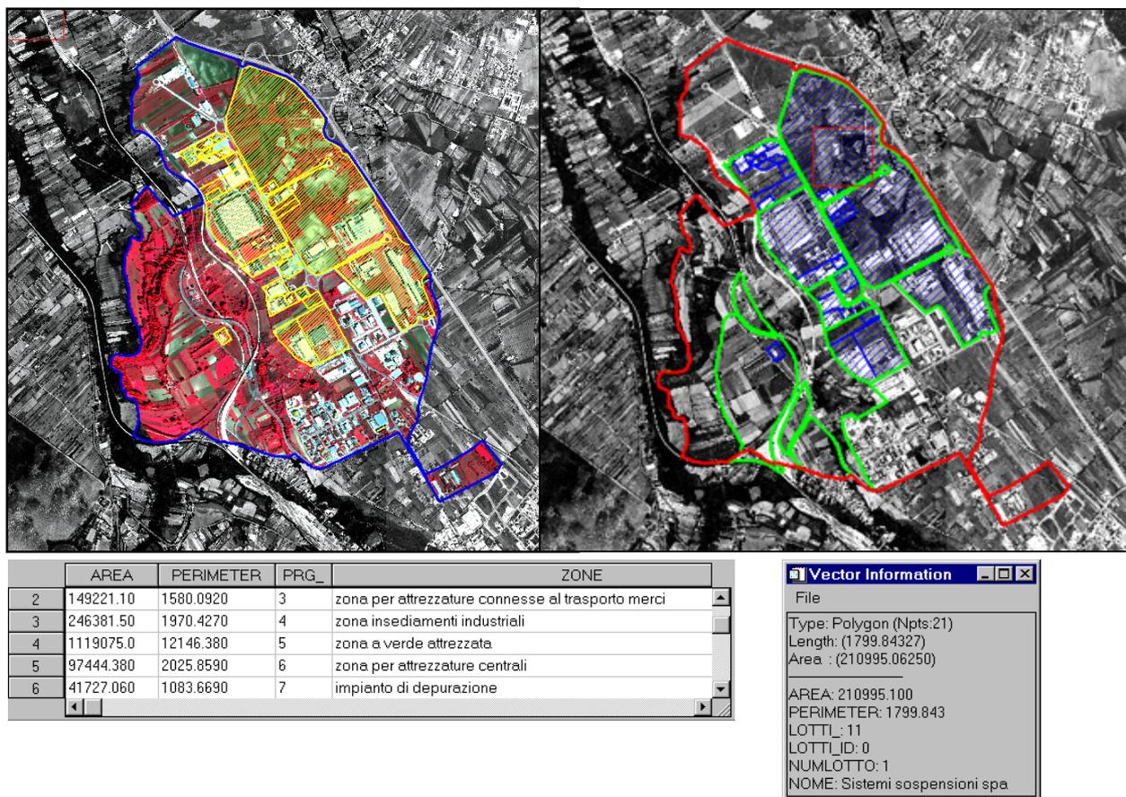
**Figure 4.** Registration of quantitative and qualitative information about the industrial installations (Sulmona, Italy) as raster and vector layers into the ArcView GIS®
