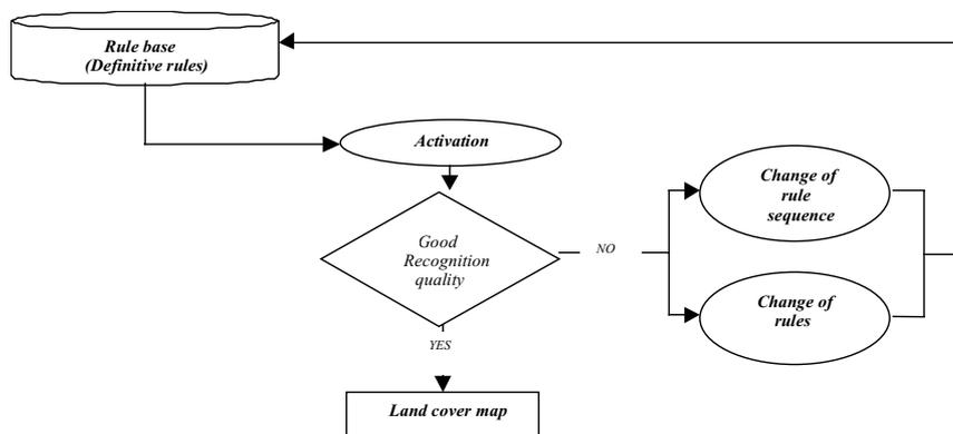
Figure 3b. Definite knowledge-based iterative classification mechanism
