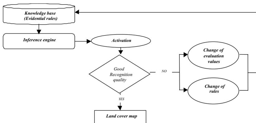
Figure 3a. Evidential knowledge-based iterative classification mechanism
