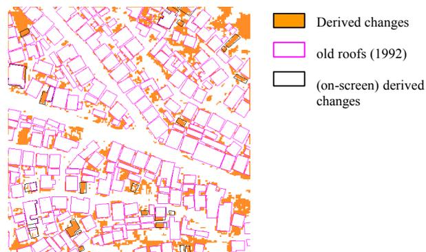
Figure 12. Derived changes from on-screen digitizing overlaid with changes from segmentation
