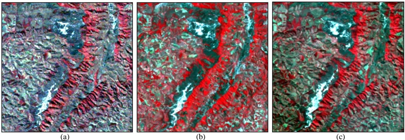
Figure 3. Landsat MSS from 1981 (a) bands 321 in RGB. Landsat TM from 1985 (b) and from 1998 (c) bands 432 in RGB reduced to 60 m of ground resolution. Using this colour combination forest areas appear in red tones while mining sites appear in white.
