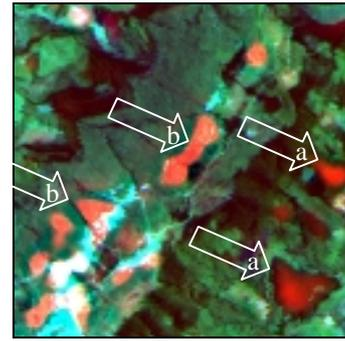
Figure 5. Landsat TM from 1985. Changes of interest coloured with red, band 4 with green and band 3 with blue. Arrows indicate areas where (a) deforestation and (b) mining increased.
