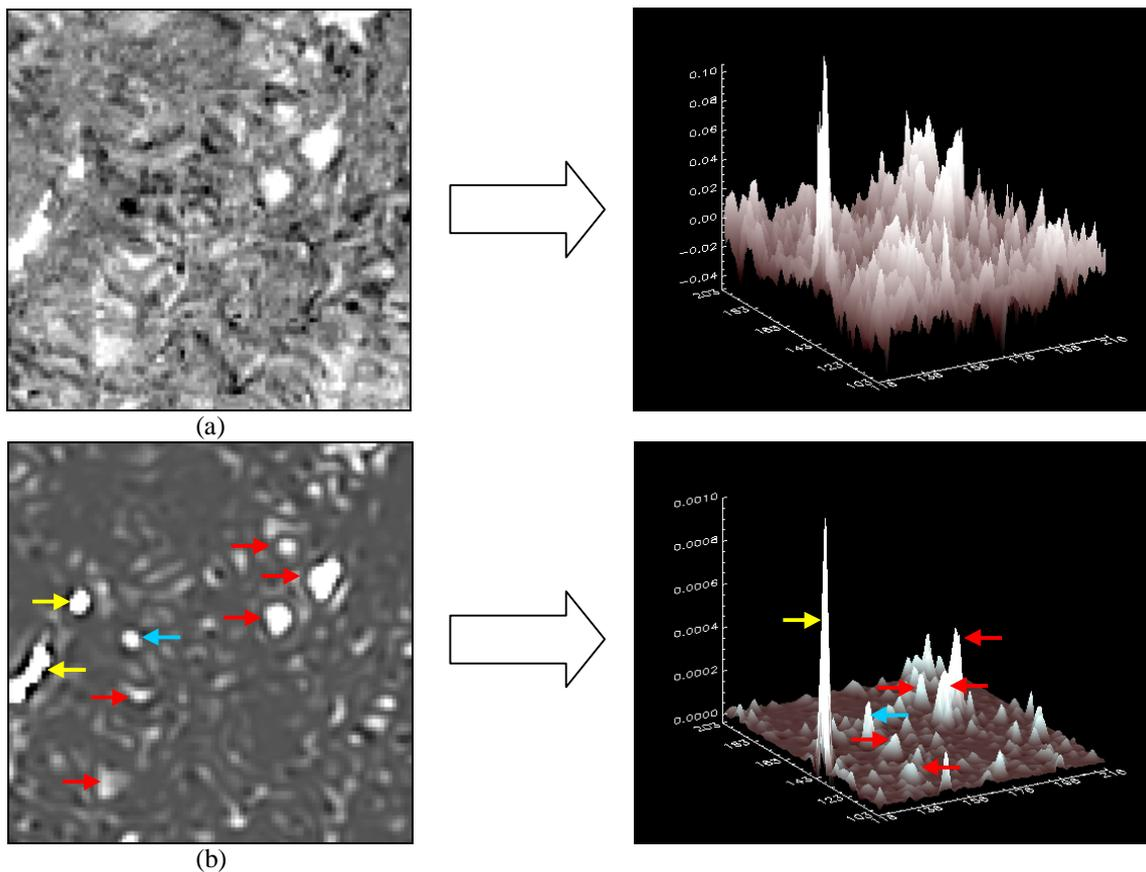
Figure 6. (a) Difference image between band 3 of Landsat TM from 1998 and band 2 of Landsat MSS from 1981 with respective magnitude graph. (b) Product of differences at second and third scales and respective magnitude graph.
