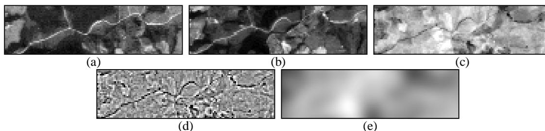
Figure 7. Landsat TM from (a) 1998 and (b) 1985 and (c) respective difference image. (d) Details of the difference image at the first scale level. (e) Smoothed version of the difference image at the fourth scale level. Note the misregistered road depicted in (d) while overall differences like phenological condition of vegetation patches are depicted in (e).
