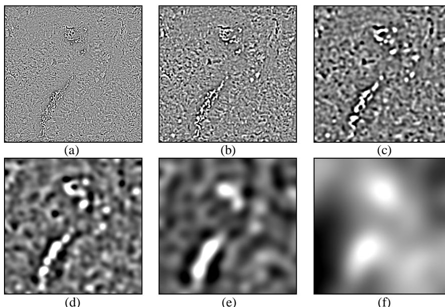
Figure 4. Detail images ranging from fine to coarse (a, b, c, d and e) and smoothed version (f) of the difference between 1998 (TM band 3) and 1981 (MSS band 2) decomposed using the *à trous* algorithm.
