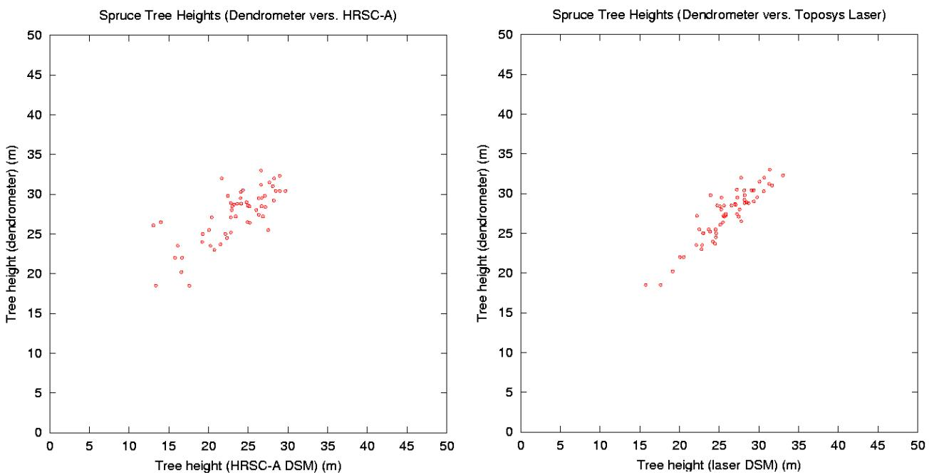
Figure 4: Scatterplot of dendrometer (ground based) measured tree heights and HRSC-A and TopoSys laser (DSM) measured tree heights of spruce trees (forest of Tharandt).
