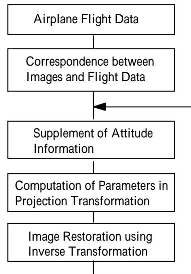
Fig. 3 General Flow for Restoration of Images Distorted by Flight Dynamics
