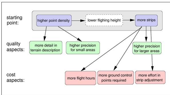
Figure 13. Consequences of higher point density.
