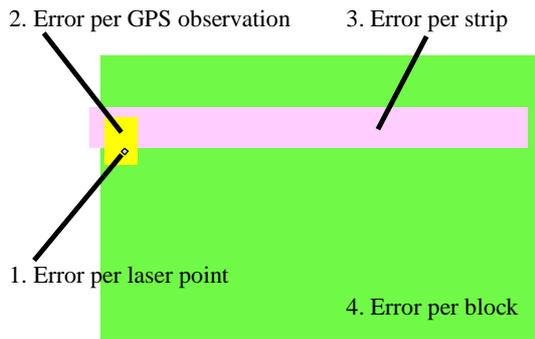
Figure 7. Error components of laser altimetry and their spatial resolution.
