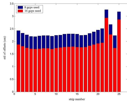
Figure 10. Standard deviations of strip offsets from strip adjustment with 8 (blue) and 16 (red) ground control points.
