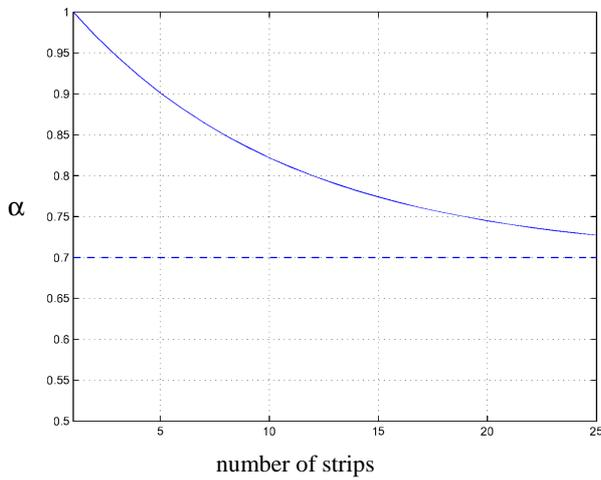
Figure 12: Scale-factor  $\alpha$  depending on the number of strips for case 2 ( $2 < n_{gcp}/n_{cross} < 5$ )
