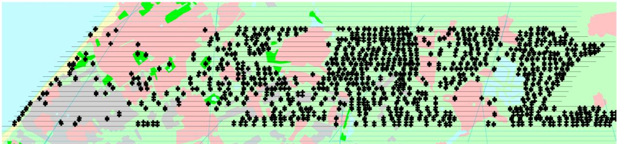
Figure 6. Locations of the 1612 tie points in the test area.
