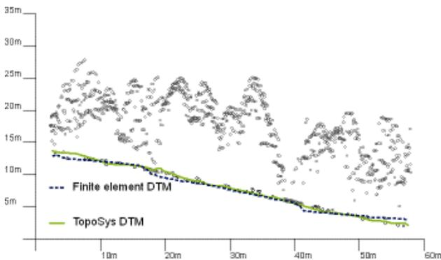
Figure 5. Filtered DTM in profile (sub area C3)
