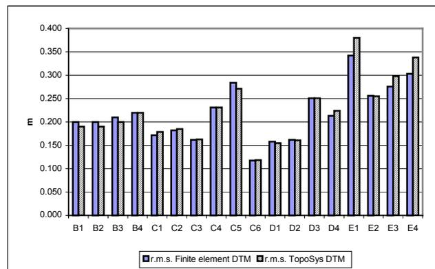
Figure 4. DTM Standard deviation of sub areas
