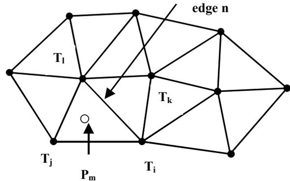
Figure 2. TIN DTM
