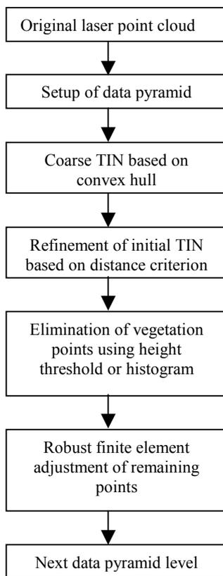
Figure 1. Scheme of laser filtering process
